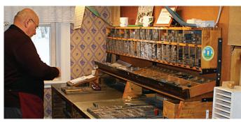
▲ The work benches are of the "newer" model, with flat work surfaces. In the early 1920s they replaced the tilted work benches (on display in our exhibition hall) for hand composing longer texts (ox setting) was replaced by machine composers. The benches are called shelves and contain a number of drawers for storing different fonts.
