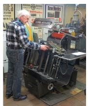
◀ The Heidelberg Press, commonly called "the Wing", is most likely the best-selling press in the world. The basic construction was finished as early as 1914, but continuous improvements were made later. The press was manufactured in Germany until 1985 and then for a while in Czechoslovakia. It is still in use at many printing houses around the world. This press is our only automatic press, where the paper is fed in and out automatically.
